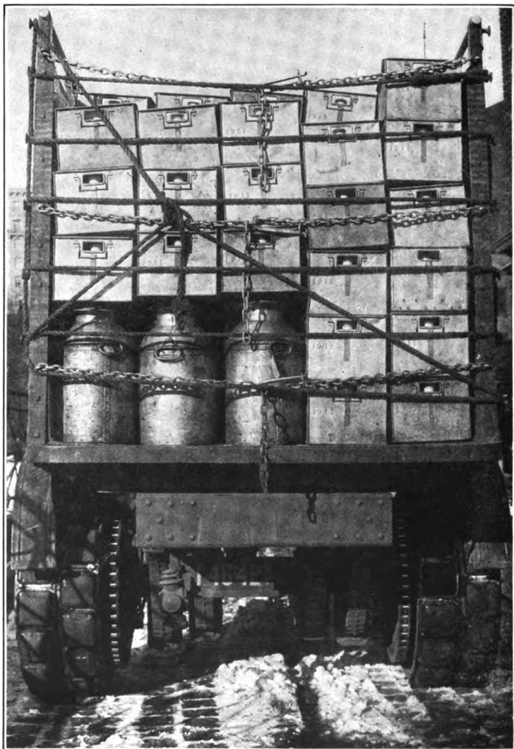
PLATE X. — Truck for hauling milk from railroad terminal to city bottling plant.
